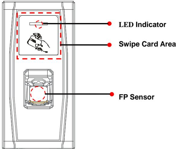
❖ **LED indicator:** The LED indicator is used to display device operation results and exceptional statuses which are defined as follows:
