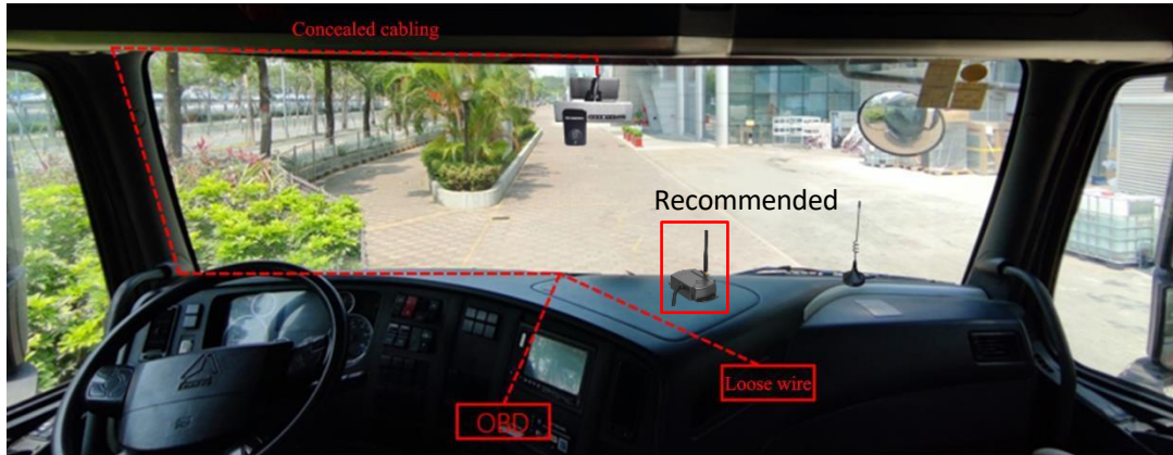
General Positions of OBD Port of Different Vehicle Models
