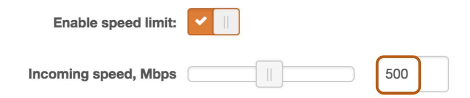
Note: speed limit is applied on both ports ETH1 + ETH2
