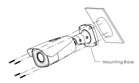
4 Bracket adjustment. Before adjustment, preview the image of the camera on a monitor and then loosen the fixed screws to adjust the view angle of the camera. After that, tighten the fixed screws.
