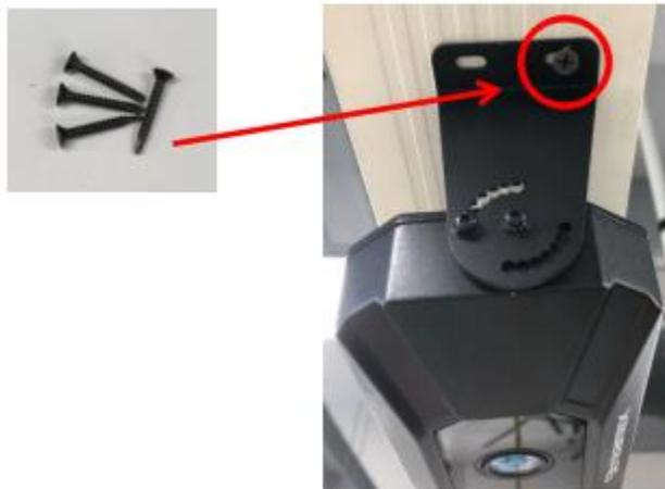
3. Adjust the pitch angle so that it is horizontal and the lens is vertical to the pedal area. Then fix MDVR-PCC2 by screw.
