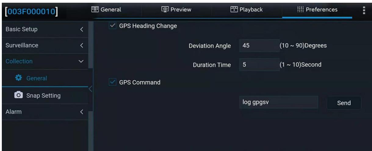
After the "log gpgsv" command is sent at the same time, the general information display interface of "Veyes" displays the satellite positioning signals received by the device. By choosing **General > Positioning Information**, you can view the number of satellites and the corresponding satellite signal quality.
