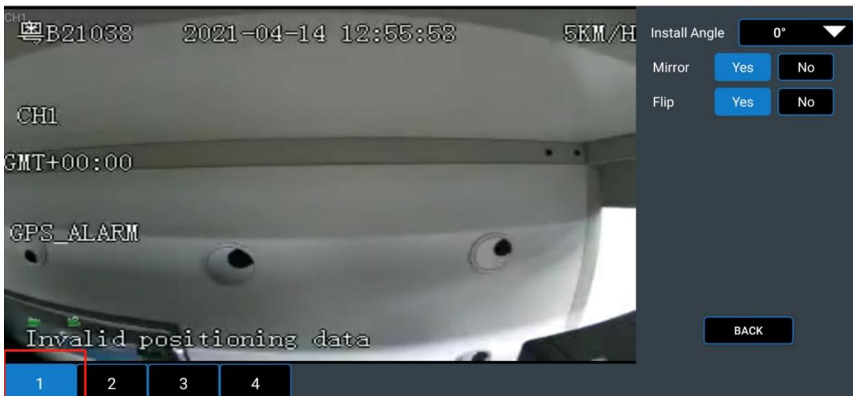
On the lower left corner of the screen, select the target channel to set the rotating angle of the camera in this channel, and enable or disable mirroring and flipping for the camera.
