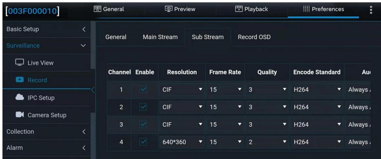
1. **Enable:** Sub-stream recording is enabled for a specific channel after this option is selected.
